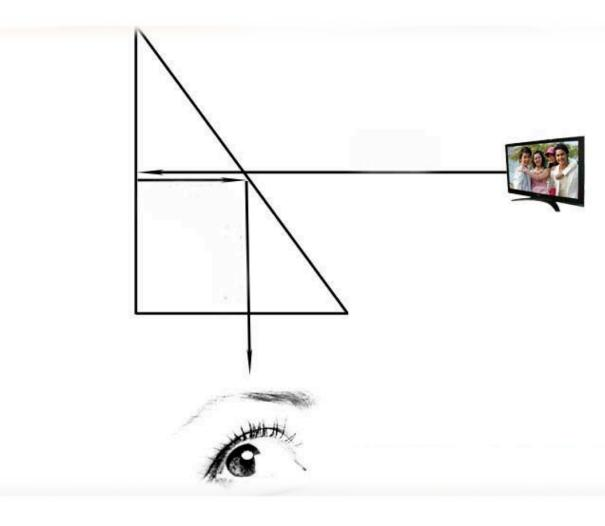
It works a little like a periscope, using mirrors to bounce light from one place to another to allow a wearer to effectively see in an unnatural direction.
